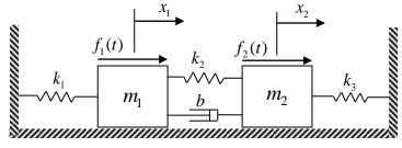
f. System #6: The forces  $f_1(t)$  and  $f_2(t)$  are the system input. The spring of stiffness  $k_1$  is unstretched when  $x_1 = x_2$ , and the spring of stiffness  $k_2$  is unstretched when  $x_2 = 0$ .
