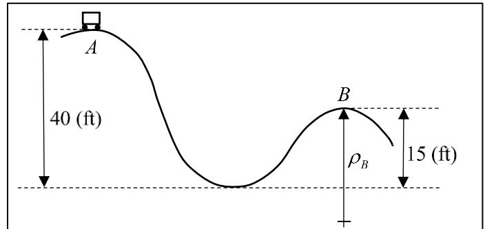
c)  $(\rho_B)_{\min}$  the **minimum radius of curvature** of the track at  $B$  so the cart does not leave the track.
