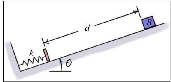
Find: a)  $v$  the velocity of the block **just before** it hits the spring, and b)  $e_{\max}$  the maximum deflection of the spring. Neglect the size of the block and the work done by the weight and friction forces during the compression of the spring.
