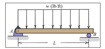
O To find the *internal forces* and *moments* acting on any *cross section* of the beam, it is *cut* at that point to *expose* them. The diagrams below show the beam cut at a distance x from the left end. As the diagram indicates, the beam experiences a *shear force* V and a *bending moment* M at that point. Note that they are shown equal and opposite on the two sections in compliance with Newton's third law.
