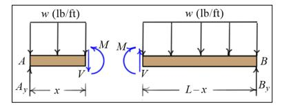
The *shear force V* and *bending moment M* can be found by writing the *equilibrium equations* for either of the two free body diagrams. The *distributed loads* over each section can be replaced by single concentrated load on that section. See the diagram below.
