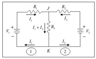
$$\sum_{\text{loop 1}} (\text{voltage rises}) = V_1 = \sum_{\text{loop 1}} (\text{voltage drops}) = R_1 I_1 + R_3 (I_1 + I_2)$$
