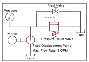
Fig. 1: Circuit diagram for the motor, pump, tank, vent valve, and relief valve.
