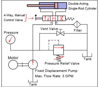
Figure 4: Simple actuation circuit with a doubleacting cylinder and manual 4-way valve.
