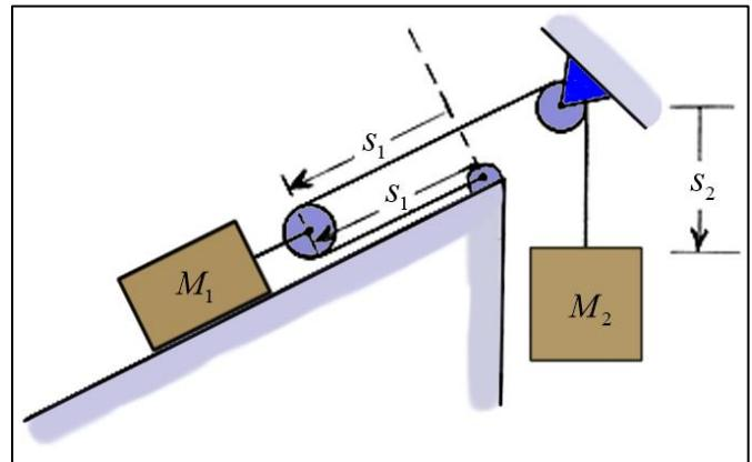
Note that  $2s_1 + s_2$  *does not represent* the *total length* of the cable; however, the only lengths that are left unaccounted for are all constant. So, the length  $2s_1 + s_2$  itself must be constant.
