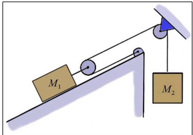
To write the “*no-stretch*” condition for this system, we first define the *distances*  $s_1$  and  $s_2$  as shown. Note that these distances not only measure lengths of certain portions of the cable, but they also measure the motion of the two masses relative to fixed reference positions. The “*no-stretch*” condition of the cable can then be written as
