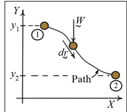
The work is **positive** when the particle moves **down** and **negative** when it moves **up**.
