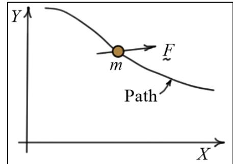
An integrated form of Newton's second law can be developed relating the **work done** on the particle to the change in its **kinetic energy** as follows:
