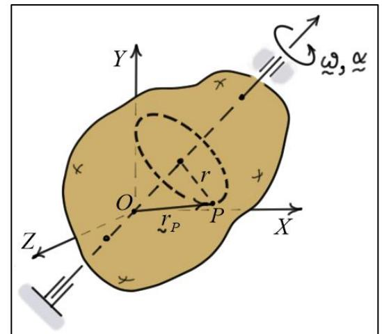
$$\underline{v}_P = \underline{\omega} \times \underline{r}_P \quad \text{and} \quad \underline{a}_P = (\underline{\alpha} \times \underline{r}_P) + \underline{\omega} \times (\underline{\omega} \times \underline{r}_P)$$
