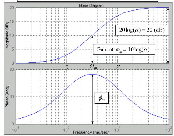
O Here,  $\alpha = 10$ , the *logarithmic mean frequency* is  $\omega_m = \sqrt{|pz|} = 3.16$  (rad/s), the overall magnitude increase is  $20\log(\alpha) = 20$  (dB), and the phase shift at the mean frequency is  $\phi_m = \sin^{-1}\left(\frac{\alpha-1}{\alpha+1}\right) = +54.9$  (deg).
