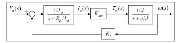
o **Block diagram reduction** gives the transfer function from the input **armature voltage** to the resulting **motor speed change**.
