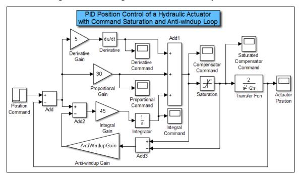
Model results are shown below for two anti-wind-up gains and a PID command signal saturation level of 20. The top two plots show the PID command signals for anti-wind-up gains of 0.025 and 0.075. The bottom two plots show the saturated command signals and the actuator position response associated with the two anti-wind-up gains.
