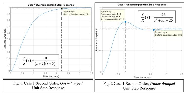
The measured percent overshoot of 16.3% is consistent with plot of percent overshoot versus damping ratio presented in earlier notes and Fig. 5.8 of the Dorf & Bishop text. The plot from previous notes is reproduced here for convenience of the reader. See Fig. 3 below.
