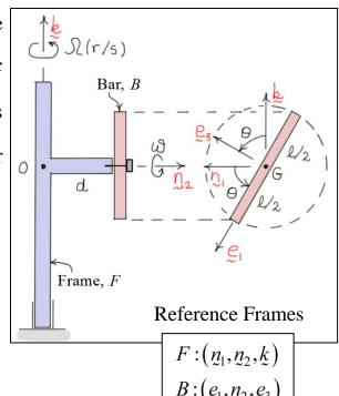
The equations of motion of B can be found by applying the *Newton/Euler equations* to the free-body diagrams shown at the right.
