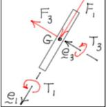
Given the angular rate  $\Omega$  = constant, the terms on the right side of the moment equation can be calculated as follows.
