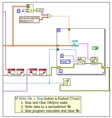
Fig. 6. Segment to Record Data and Stop Execution
