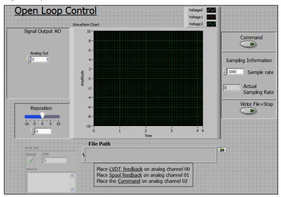
Fig. 1. The Front Panel (Graphical User Interface)
