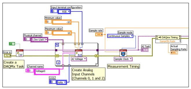
Fig. 2. Segment to Create DAQmx Task and Initialize Analog Input Channels
