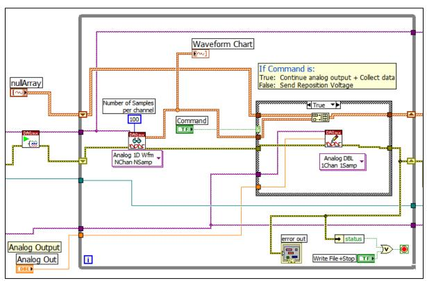
Fig. 5. The Data Acquisition Segment with the Command Button ON
