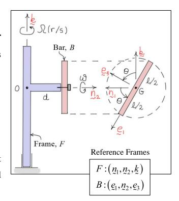
Assuming the degrees of freedom of the system are described by the *generalized coordinates*  $\phi$  ( $\dot{\phi} = \Omega$ ) and  $\theta$ , the *equations of motion* of the system can be found using Lagrange's equations shown in Eq. (1).
