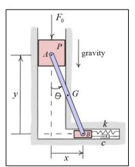
2) Show that  $x = \theta = 0$  is an equilibrium position for the system of Exercises #8, problem #2. Linearize the equations of motion about this position and calculate the natural frequencies and mode shapes of the system using the following physical data. Describe the motion of each mode.
