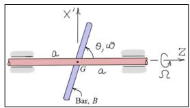
4) Given that  $M_{\theta}=0$ ,  $\dot{\phi}=\Omega={\rm constant}$ , and b=0, show that the equilibrium position for the angle  $\theta$  for the bar of Exercises #8, problem #4 is approximately  $\theta_{eq}\approx 58.7$  (deg). Then linearize the equation of motion about this position and determine the stability of small motions about that position. Find the torque  $M_{\phi}$  required so that  $\dot{\phi}=\Omega={\rm constant}$ . Use the following physical data:
