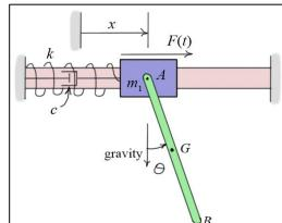
3) Given that  $M_{\theta}=0$  and  $\dot{\phi}=\Omega={\rm constant}$ , find the equilibrium positions for the angle  $\theta$  for the bar of Exercises #8, problem #3. Then linearize the equation of motion about these positions. Determine the stability of small motions about each of these positions. Find the torque  $M_{\phi}$  required so that  $\dot{\phi}=\Omega={\rm constant}$ .
