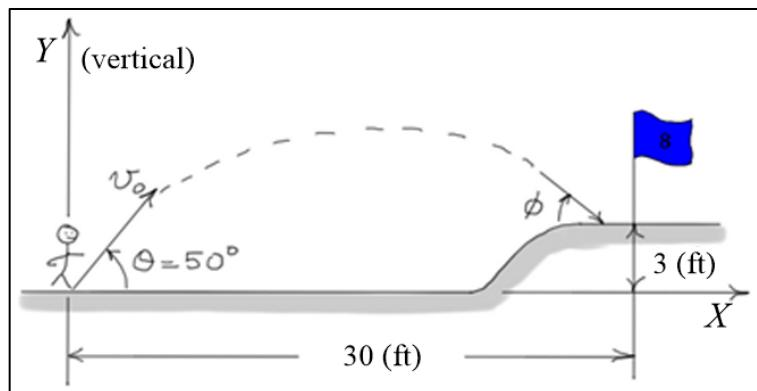
$$X \text{ direction: } x(t) = x_0 + v_{x_0} t = (v_0 \cos(50))t \quad \text{constant velocity in } X \text{ direction}$$
