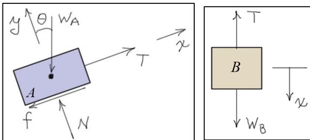
**Free body diagrams for motion or motion impending up the plane**
