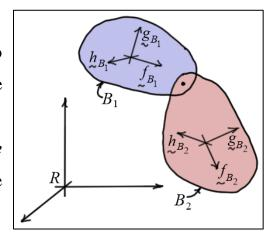
Consider the two bodies shown in the diagram. Let  $h_{B_i}$  be a vector fixed in body  $B_i$  parallel to the hinge joint, and let  $f_{B_i}$  and  $g_{B_i}$  be vectors fixed in  $B_i$  that are **perpendicular** to the hinge axis (and, hence,  $h_{B_i}$ ). The *rotational constraint* can then be expressed directly in terms of the angular velocities as follows
