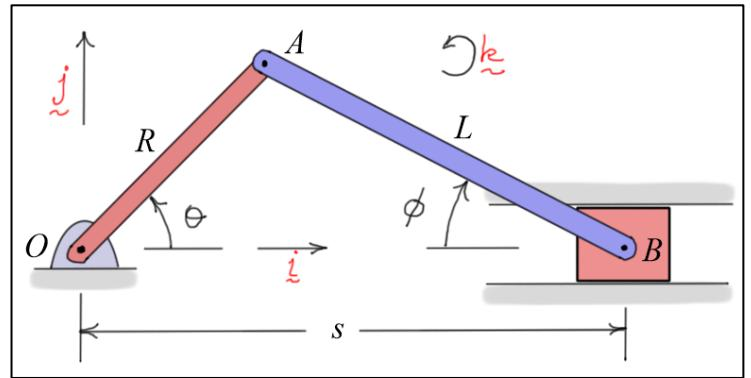
$$R \sin(\theta) = L \sin(\phi) \Rightarrow \phi = \sin^{-1} \left( \frac{R \sin(\theta)}{L} \right)_{\theta=30 \text{ (deg)}} = 14.4775 \text{ (deg)}$$
