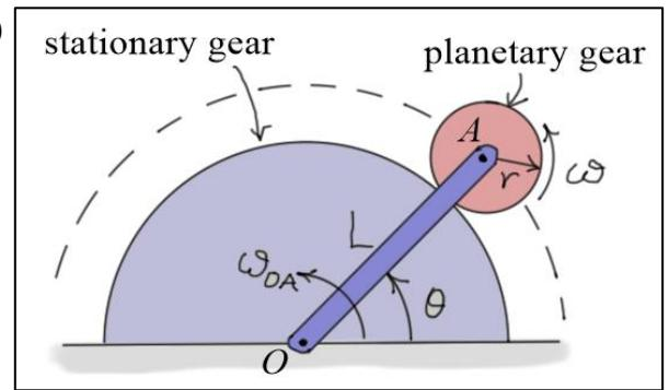
The instantaneous center of the planetary gear is at the contact point with the stationary gear. So, as the planetary gear rolls on the surface of the stationary gear, the velocity of  $A$ , the center of the gear, can be written as
