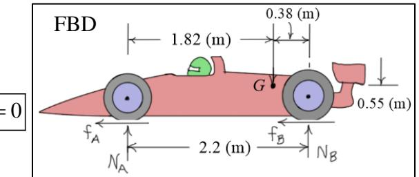
Substituting into the moment equation for the friction forces in terms of the normal forces, the last two equations can be solved for the normal forces.
