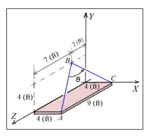
$$\underbrace{\left[ \underbrace{u_{AB}} = \left( -4 \underbrace{i} + 4 \underbrace{j} - 7 \underbrace{k} \right) \middle/ \sqrt{4^2 + 4^2 + 7^2} \right] = -\frac{4}{9} \underbrace{i} + \frac{4}{9} \underbrace{j} - \frac{7}{9} \underbrace{k}}_{CB} }$$
