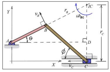
a) First, construct the dashed lines to the *instantaneous center*. Then *construct* the *right triangle ADIC*, and *calculate* the angle of *AB* relative to *AD*.
