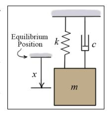
To determine which type of response a system will have, we calculate  $c_c$  the *critical damping* coefficient.
