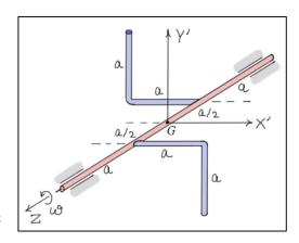
**1.5** The system shown consists of a bar B that is pinned through the center of a shaft of length 2a. As the shaft rotates about the Z-axis at a rate  $\Omega$  (r/s), B rotates about the Y' at a rate  $\dot{\theta} = \omega$  (r/s). (a) Find  $H_G$  the angular momentum of B about its mass center G. Express your results in the X', Y', and Zdirections. (b) Find *K* the kinetic energy of *B*.
