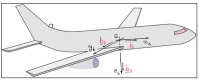
the *airframe* A and the *two engines*  $E_1$  and  $E_2$ . The term *airframe* is used to refer to all the *stationary components* of the aircraft, and the term *engine* is used to refer to the *rotating components* of the engines. The points  $G_i$  (i = 1, 2) are the mass centers of the two *engines*,  $G_A$  is the mass center of the *airframe*, and G is the mass center of the *aircraft*.
