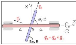
Find the equations of motion for the system of Exercise 5.3 using Kane's equations assuming the shaft is light. Use  $(u_1, u_2) = (\omega_1, \omega_2) \triangleq ({}^R \omega_B \cdot e_1, {}^R \omega_B \cdot e_2)$  as the two independent generalized speeds.
