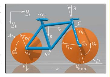
The steering column is assumed to be tilted relative to the vertical at an angle  $\lambda$ . This angle is a right-hand rotation about the  $N_2 = N_3 \times N_1$  direction. The projection of the steering axis onto the horizontal plane is assumed to be a distance c in front of the contact point Q. Positive rotations of the front and rear wheels are also measured about the  $N_2$  direction, so for forward motion of the bicycle, both angles  $\theta_F$  and  $\theta_R$  are **negative**.
