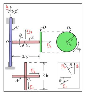
Using Kane's equations, find the equations of motion for the system. Use  $(u_1, u_2, u_3) = (\omega_1, \omega_2, \omega_D) \triangleq ({}^R \omega_A \cdot n_1, {}^R \omega_A \cdot n_2, {}^A \omega_D \cdot n_2)$  as the three independent generalized speeds.
