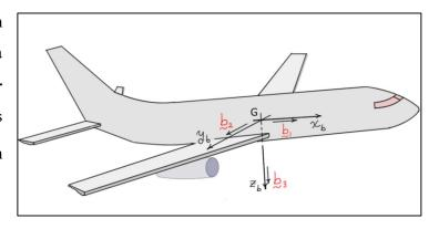
The term *airframe* is used to refer to all the *stationary components* of the aircraft, and the term *engine* is used to refer to the *rotating components* of the engines. The points  $G_i$  (i = 1, 2) are the mass centers of the two *engines*,  $G_A$  is the mass center of the *airframe*, and G is the mass center of the *aircraft*.
