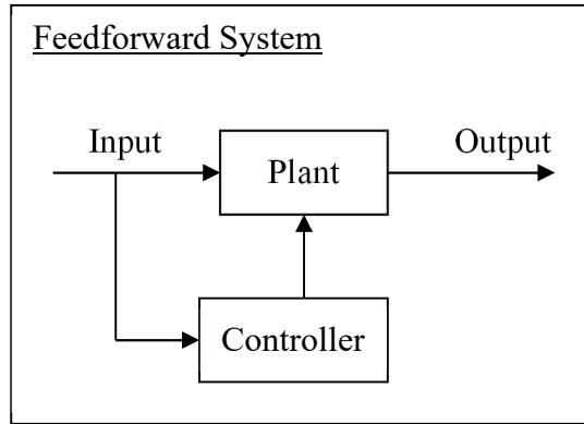
If the behaviour of a plant is **linear**, that is, if it can be described using a **linear algebraic** or a **linear differential** equation, then the plant can be described using a **transfer function**, indicated by  $G(s)$  in the diagram below. The purpose of a transfer function is to provide an **accurate quantitative representation** of the output of the plant given its input. Transfer functions associated with linear differential equations can be found using **Laplace transforms**.
