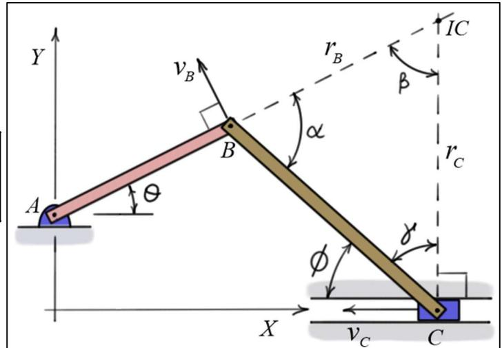
b) Construct the dashed lines to the **instantaneous center**. In the newly constructed triangle  $BCIC$ , define the **unknown angles**  $\alpha$ ,  $\beta$ , and  $\gamma$ .
