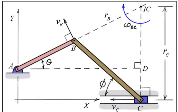
a) First, construct the dashed lines to the **instantaneous center**. Then **construct** the **right triangle**  $ADIC$ , and **calculate** the angle of  $AB$  relative to  $AD$ .
