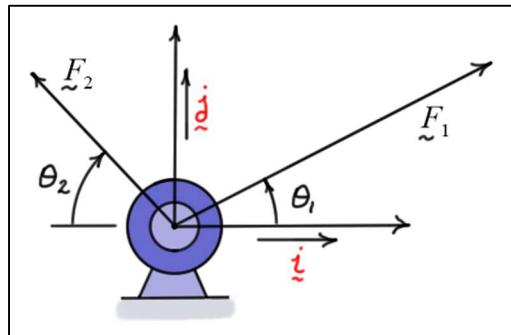
a) The **total force**  $\underline{F}$  acting on the support in terms of the unit vectors shown.
