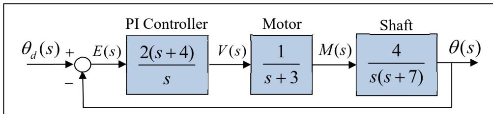
c) Using block diagram reduction, with  $G = N_G/D_G$  and  $H = 1$
