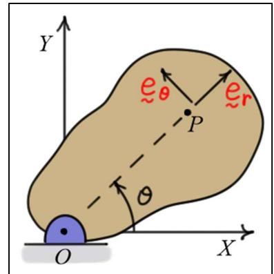
Here,  $\theta$  is measured ***counterclockwise*** relative to a ***fixed horizontal line***. The velocity and acceleration of point  $P$  can be computed as
