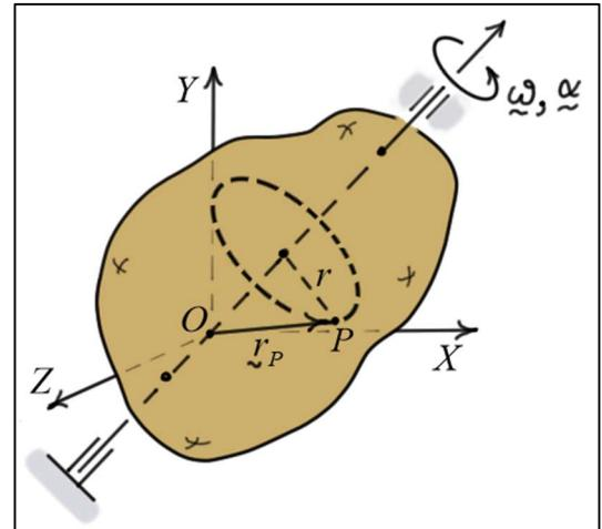
$$v_P = \underline{\omega} \times \underline{r}_P \quad \text{and} \quad \underline{a}_P = (\underline{\alpha} \times \underline{r}_P) + \underline{\omega} \times (\underline{\omega} \times \underline{r}_P)$$
