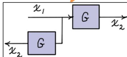
6. Collapsing a feedback loop:
