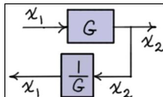
5. Moving a pick-off point in front of a block:
