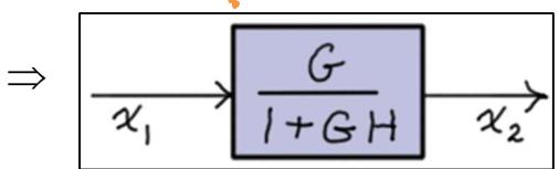
As shown, the system is said to have “**negative feedback**”, because the signal  $x_3$  is **negated** at the summing block. If the system has “**positive feedback**”, then it is easy to show that the transfer function becomes
