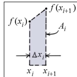
So far, we considered the function  $f(x)$  and the increments  $\Delta x_i$  to be **positive**. Consequently, the area  $A$  is **positive**. If, however,  $f(x)$  is **negative** over this range the area will be **negative**. Clearly, if  $f(x)$  takes on both **positive** and **negative** values, the resulting area could be **positive**, **negative**, or **zero**.
