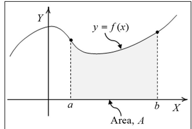
In this form, the integral is called a **definite integral**. It is a **number**, not a function. Later, we will define an **indefinite integral** which is itself a **function** of  $x$ .
