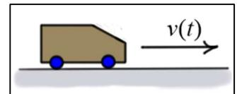
$$s = \int_{t_1}^{t_2} v(t) dt$$
