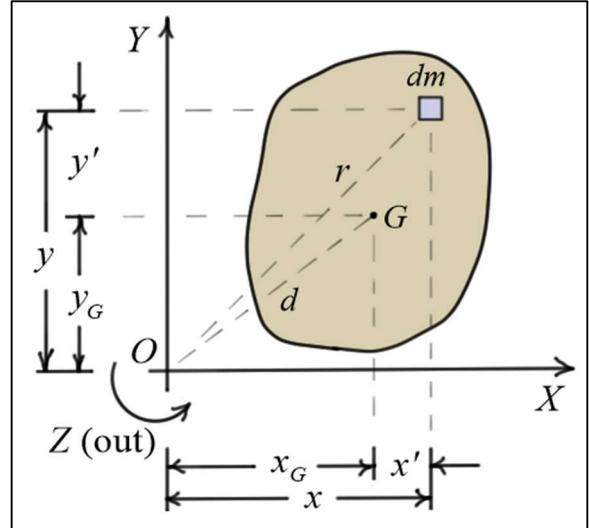
The **larger** the inertia, the **further** the mass is spread away from the axis. The **smaller** the inertia, the **closer** the mass is located to the axis. The units of  $I_Z$  are **slug-ft<sup>2</sup>** or **kg-m<sup>2</sup>**.
