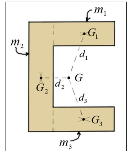
Here,  $I_{G_i}$  represents the moment of inertia of the  $i^{\text{th}}$  component shape about its own mass center  $G_i$  and can be found in the tables for common geometric shapes.
