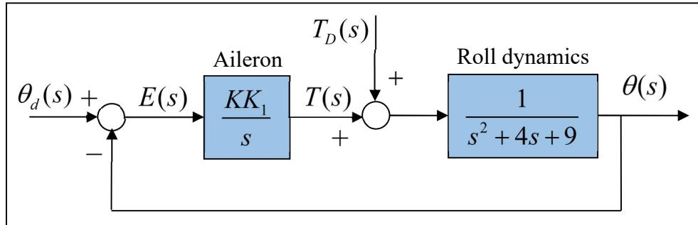
The variables  $\theta_d(s)$  and  $\theta(s)$  represent the **desired** and **actual** roll angles of the aircraft, and the variable  $T_d(s)$  represents a **disturbance roll torque** on the aircraft. **Question:** Are there **reasonable values** of the **product**  $KK_1$  that allows the system to have a **desirable response** to step commands in roll angle and to maintain **small roll angles** in the presence of a disturbance?
