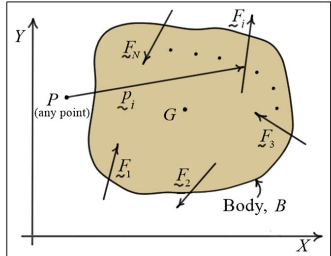
Note the term  $\tilde{r}_{G/P} \times m \tilde{a}_G$  is added to the right side of the moment equation and represents the moment of vector  $m \tilde{a}_G$  about point  $P$ . The line of action of  $m \tilde{a}_G$  is assumed to pass through  $G$ .
