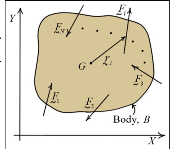
Here,  $(\tilde{M}_G)_i$  represents the **moment** of force  $\tilde{F}_i$  about the **mass center**  $G$ , and  $I_G$  represents the **moment of inertia** of the body about a  $Z$  axis passing through  $G$ .
