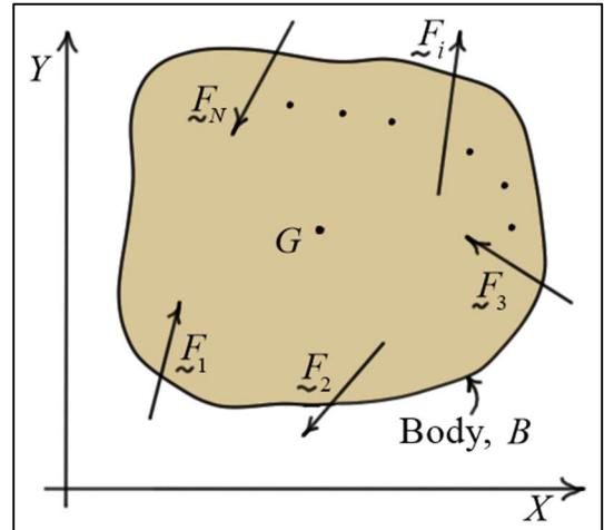
Here,  $U_{1 \rightarrow 2}$  represents the **work done** by all the forces and torques acting on the body as it moves from position 1 to position 2, and  $KE_i$  ( $i=1,2$ ) represent the kinetic energies of the body in those two positions.
