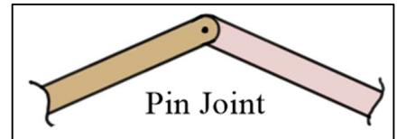
However, the **net work** done on the system of the two members is **zero**, because the pin forces on the members are equal and opposite and move through the same displacement.
