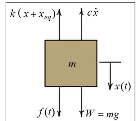
$$\boxed{\dot{x}(t) = v(t) = Ase^{st} \Rightarrow \ddot{x}(t) = a(t) = \frac{dv}{dt} = \frac{d}{dt}(Ase^{st}) = As^2 e^{st}}$$
