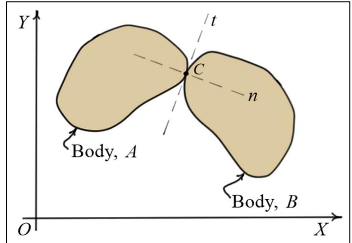
$$e = \frac{(v_{CB})_{n2} - (v_{CA})_{n2}}{(v_{CA})_{n1} - (v_{CB})_{n1}}$$
