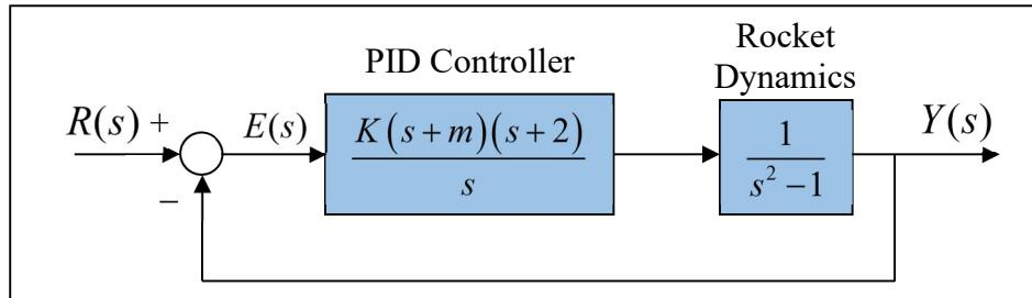
Here,  $R(s)$  and  $Y(s)$  represent the **desired** and **actual attitude angles** of the rocket (assuming the rocket moves in a vertical plane). Note that the rocket dynamics are **unstable**, because the poles are at  $\pm 1$ .
