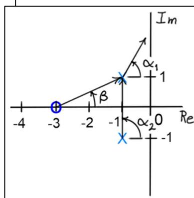
4. Sketch the root locus diagram for the parameter  $K$  for the closed loop system shown in the diagram.
