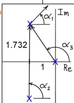
3. Sketch the root locus diagram for the parameter  $K$  for the closed loop system shown in the diagram.
