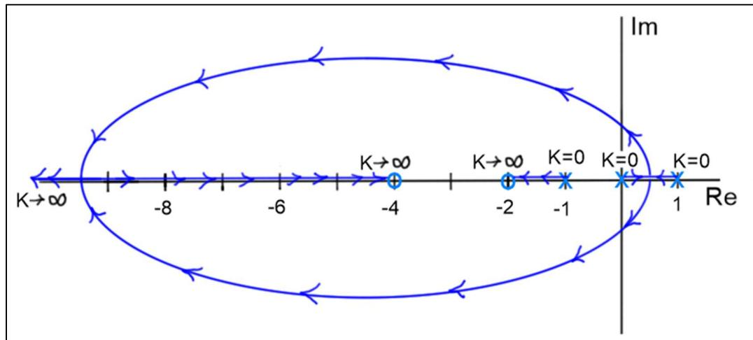
6. Sketch the root locus diagram for the parameter  $a$  for the closed loop system shown in the diagram.
