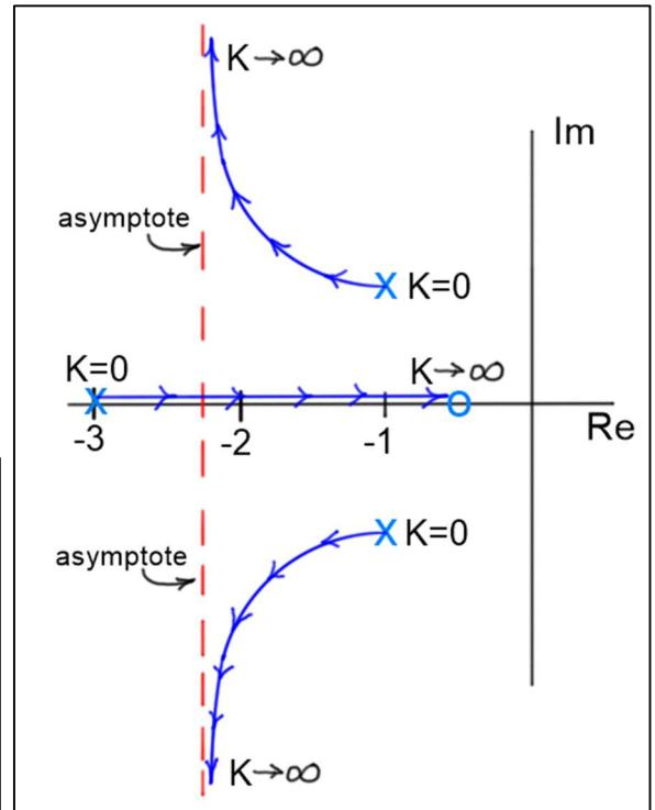
5. Sketch the root locus diagram for the parameter  $K$  for the closed loop system shown in the diagram.
