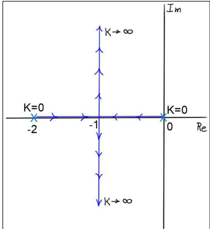
2. Sketch the root locus diagram for the parameter  $K$  for the closed loop system shown.
