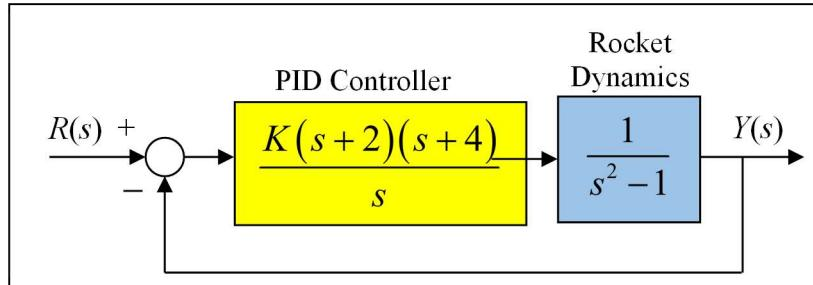
The **characteristic equation** of the closed-loop system is  $1 + GH(s) = 0$  or  $1 + KP(s) = 0$ .
