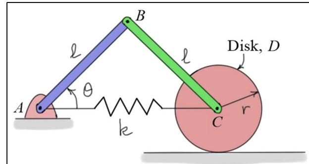
Find:  $\omega_{AB}$  the angular velocity of  $AB$  at  $\theta = 0$  (deg)
