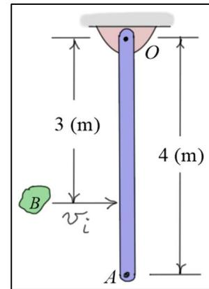
$$\oint (\underline{H}_O)_1 = (\underline{H}_O)_2 \quad (\text{state 1: just before impact; state 2: just after impact})$$
