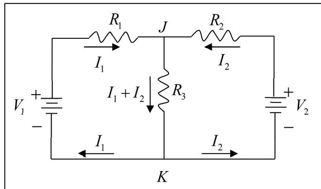
Given the resistances  $R_1 = 8(\Omega)$ ,  $R_2 = 10(\Omega)$ , and  $R_3 = 5(\Omega)$ , and the voltages  $V_1 = 12$  (volts), and  $V_2 = 24$  (volts), find the currents  $I_1$  and  $I_2$  using (a) Gaussian elimination (substitution), (b) Cramer's rule, and (c) matrix inversion. Compare the results.
