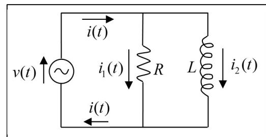
Given that  $i(t) = i_1(t) + i_2(t)$ , find  $i(t)$ . Express  $i(t)$  in the form of a single, phase-shifted cosine function.
