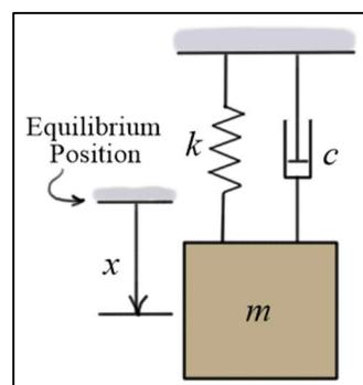
4. A spring-mass-damper system with  $m = 0.4$  (slugs),  $k = 100$  (lb/ft), and  $c = 20$  (lb-s/ft) is shown in the diagram. The system is given an initial displacement  $x_0 = 0.5$  (ft) and initial velocity  $v_0 = 10$  (ft/s).
