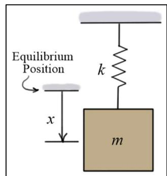
3. A spring-mass-damper system with  $m = 0.4$  (slugs),  $k = 100$  (lb/ft), and  $c = 3$  (lb-s/ft) is shown in the diagram. The system is given an initial displacement  $x_0 = 0.5$  (ft) and initial velocity  $v_0 = 10$  (ft/s). (a) Calculate  $c_c$  the critical damping coefficient, (b) Find the displacement function  $x(t)$ . Express  $x(t)$  as an exponential function times a single, phase-shifted sine function.
