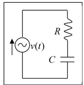
Given that  $v(t) = v_R(t) + v_C(t)$ , find  $v(t)$ . Express  $v(t)$  in the form of a single, phase-shifted cosine function.
