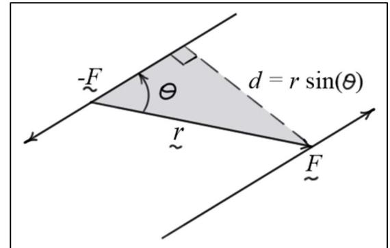
Here,  $\underline{r}$  is the **position vector** from **any point** on the **line of action** of one of the forces to **any point** on the **line of action** of the other force.
