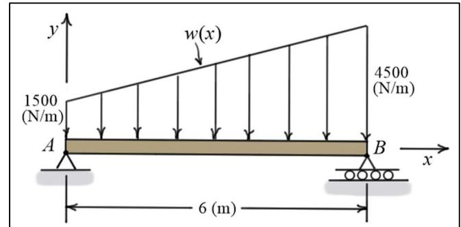
For the purpose of finding the resultant and its location, the applied load can be thought of having two parts, a constant distributed load of 1500 (N/m) and a triangular distributed load which increases from zero at  $A$  to 3000 (N/m) at  $B$ .
